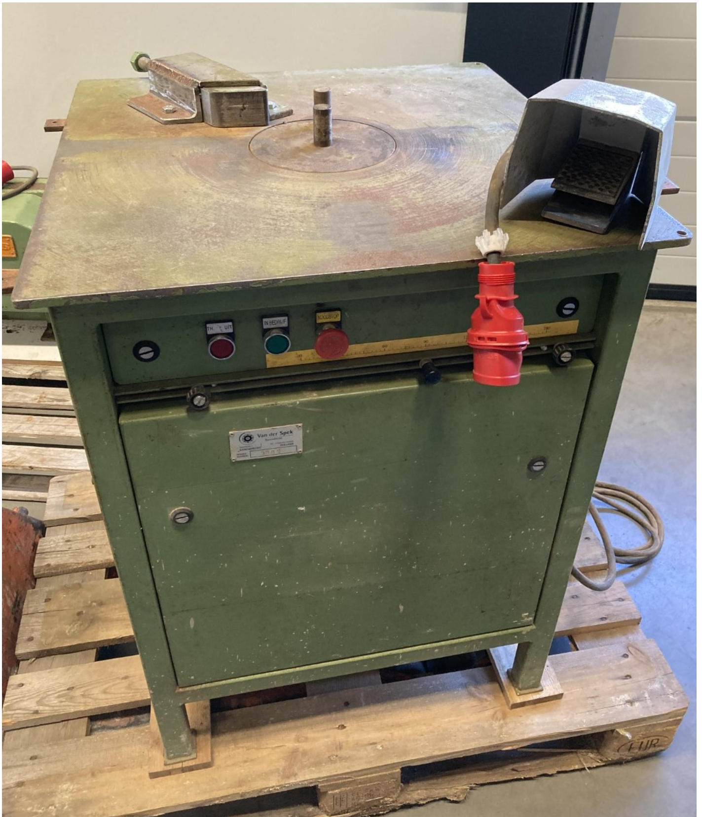
Used rebar bender model LB20, max Ø16mm
