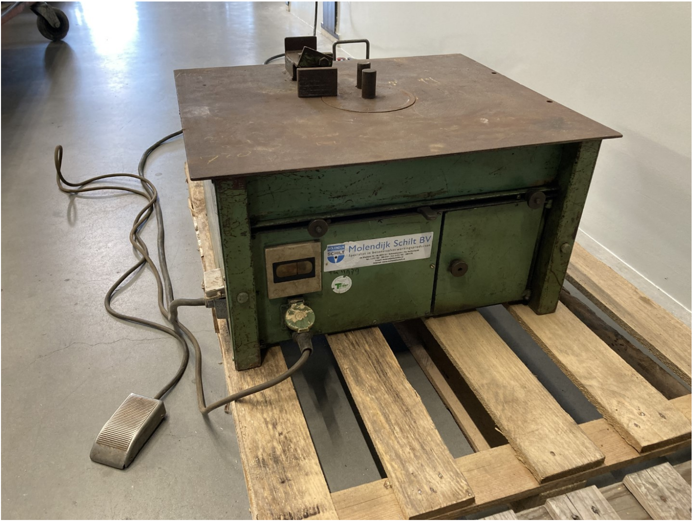
Used rebar bender model LB12, max Ø12mm
